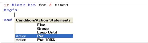
After pressing the enter key, the word <u>Put</u> is added to your system. Now again press the F2 key. This will display the next set of valid identifiers. Locate and select the **numeric data** identifier, then press the enter key. The system will insert a <u>1</u> next to the <u>Put</u> action command. At this point, manually change the numeric value from <u>1</u> to <u>5</u>.
